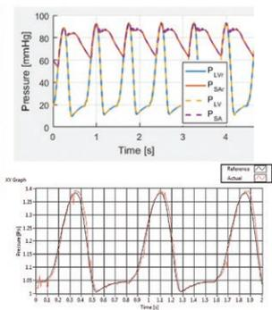
Fig 2: Tracking of left-ventricular and aortic pressure by a simulated hybrid MCL (top) and example LV pressure tracking curves in experimental testing (bottom)
