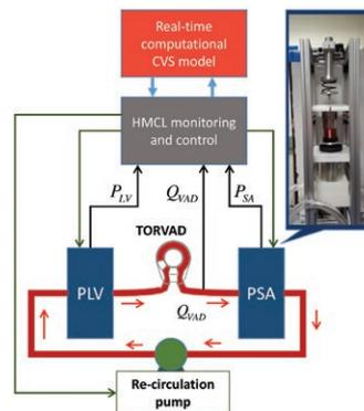
Fig 1: Hybrid MCL system schematic with insert showing prototype pressure-generating interface
